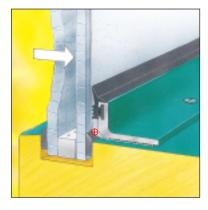
**Step Two:** Blast impact shatters external glass and drives it against the inner pane.
