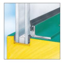
**Step One:** Madico FrameGard<sup>™</sup> secures the film tightly in place to the window frame.
