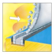
**Step Two:** Untreated edge of glass breaks and separates at the unfilmed edge of the glass.
